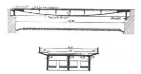
Figure 7 Prestressing system designed by Franz Dischinger in 1934 (Cestelli Guidi 1947)
